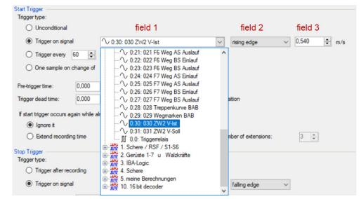
You can use analog signals and digital signals as triggers. Select the signal to be triggered via the signal tree in the selection list in field 1.
